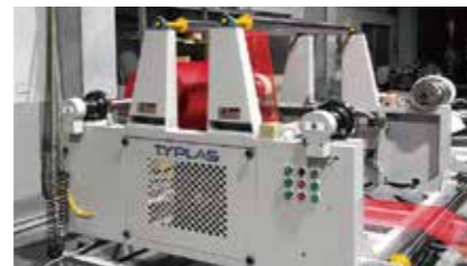
Unwinder configured with missing cloth detection and automatic unwinding change device, it makes the operation more convenient.
