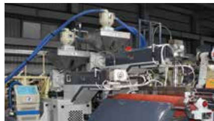
Dual extruder and dual T-die design make the operation and adjustment of film position and width more easier.
