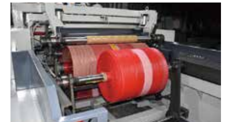
Winder configured design of auto roller changed and auto tension control to be effectively adjusted and maintain the smoothness of the cloth roll.
