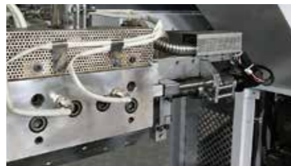
T-die servo motor automatically adjust the film, it can maintain a certain width of the film during speed acceleration or deceleration.
